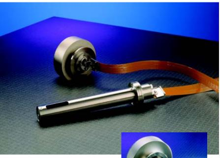
The HYT Model 20SX and Model 25SX vacuum particle sensors detect particles in non-corrosive, vacuum process equipment. These laser-based sensors can be installed in loadlock or process chambers or into exhaust pump lines. They have been proven in highproduction fabs on tools such as sputtering systems and ion implanters.
