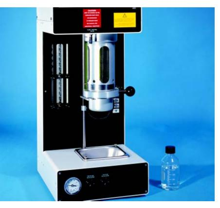
The HIAC Model ABS-2 is a pressure sampling device used for batch analysis of volatile or viscous fluids. The Model ABS-2 accurately delivers fluid to the sensor at flow rates of 10 to 200 mL/min. It contains a precision metering valve for accurate control of flow rates, regardless of sample viscosity. A check valve in the sample introduction line eliminates backflow and minimizes sample cross contamination, and an automatic drain mechanism allows unattended sample analysis of multiple runs.
