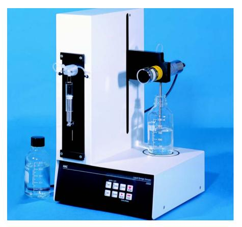
HIAC's Model 3000A batch sampler is designed to simplify your particle counting procedures. The sampler incorporates precision stepper motors for sample testing, eliminating the need for pressure lines. This means the Model 3000A can be moved and located anywhere in your lab without concern for pressure air lines.
