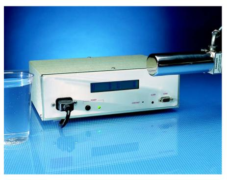
The HIAC Model 2000 provides an accurate yet inexpensive means to transfer particle data from sensor to host computer system. Up to four channels of particle size information are available. The instrument is constructed of corrosion-resistant anodized aluminum for placement in non-laboratory environments. A liquid crystal display allows the operator to view the data at the analysis site for real-time observation and decision making.
